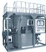
Mixing Plant YMA-25L PRODUCTION CAPACITY : 24 m 3 /hour MIXING CAPACITY : 1,000 L (264 gal) AGITATING CAPACITY : 2,400 L (634 gal) CHEMICAL DISP. CAPACITY : 45 L/min (12.8 gpm) DIMENSION(LxWxH) : 2,600 x 2,050 x 2,400 mm (8' 6" x 6' 9" x 7' 10") GROSS WEIGHT : 2,150 kg (4,740 lbs)
